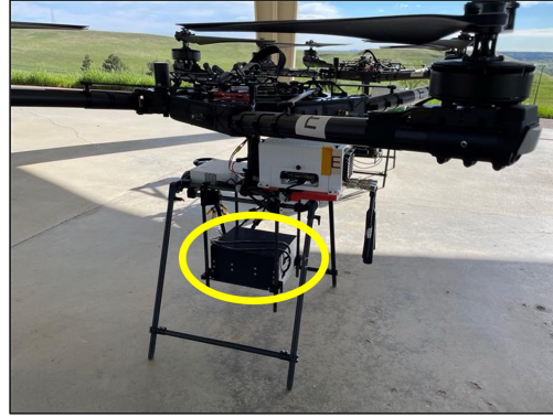
Fig. 10 The FreeFly Alta-X cargo attachment supports rapid payload integration.
