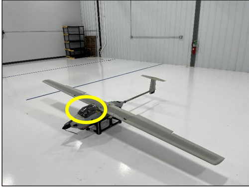
Fig. 9 The Lockheed Martin Stalker UAV supports external payload bays, shown as the black compartment on top of the nose cone.
